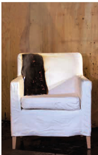
◀ Fire tests of two qualities of the same model of an upholstered armchair 5 minutes after ignition of the fire source crib 5. The photo to the left shows a chair purchased on the Norwegian market, and the photo to the right shows a chair purchased on the British market.
