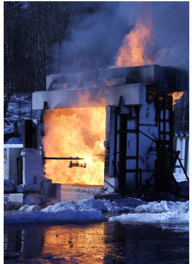
Figure 1. High heat flux jet fire test according to ISO 22899-1 with modifications.
