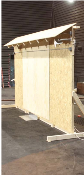
Figure 2-4 Overview of the test wall seen from the side showing the flame detector and the position of the two steel pipes holding a heat detection cable.
