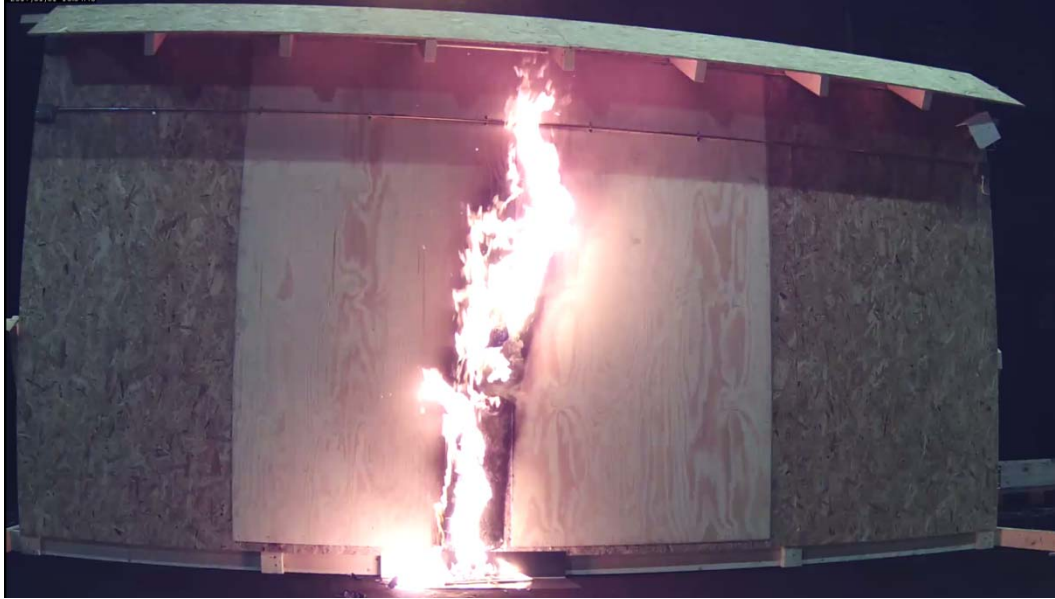
Figure 4-2 Stage of fire as the lower heat detection cable detects the fire, 7 minutes and 55 seconds after ignition.
