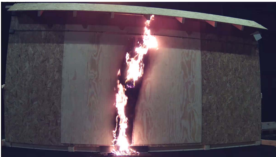
Figure 4-3 Stage of fire as the upper heat detection cable detects the fire, 8 minutes and 20 seconds after ignition.
