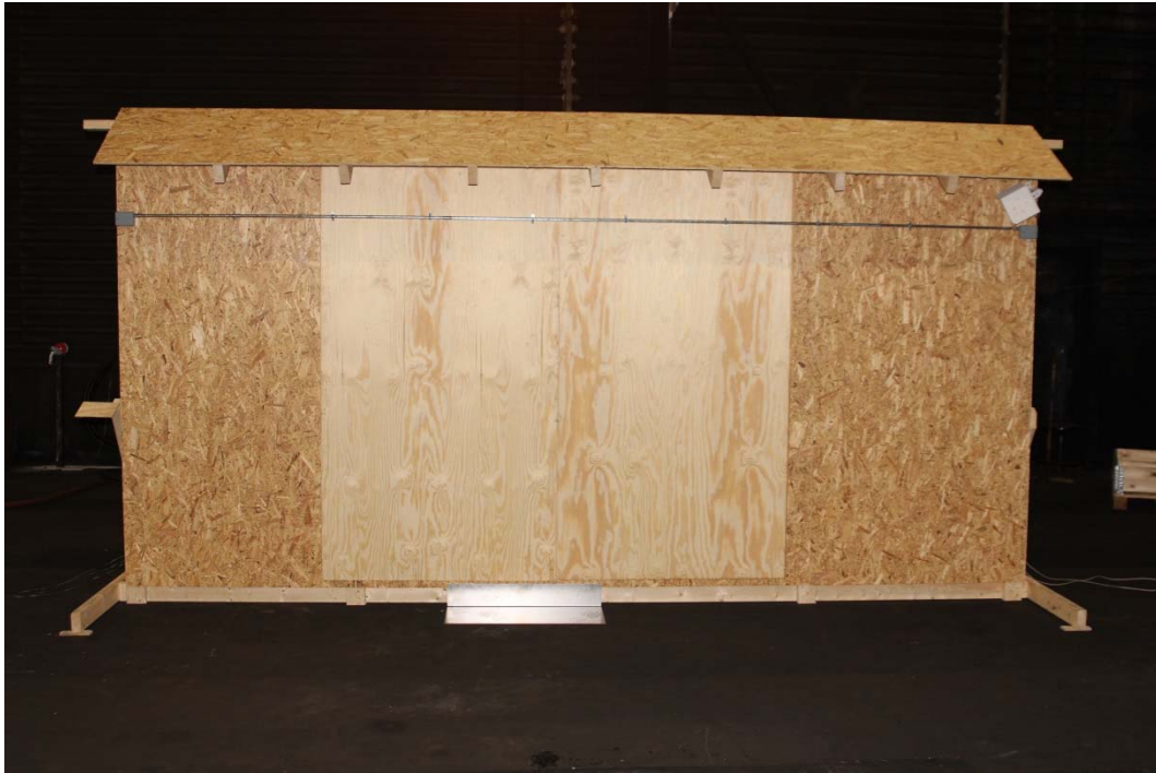
Figure 2-3 The test wall seen from the front. The flame detector can be seen in the top right corner, with the lower heat detection cable being placed in a steel pipe. The second heat detection cable is mounted under the ceiling.
