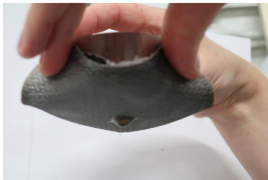
Figure 3-4 Example of droplet formation on the unexposed side of the textile, for material 5 after heat exposure of 30 kW/m 2 . The observation was made while the textile was lying in the set-up, and lifted up here only for this illustration photo.
