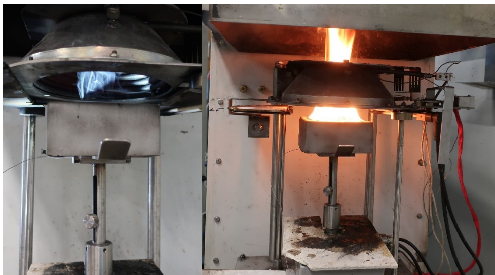
Figure 2-2 During heat exposure, visual observations of smoke (left) and of flaming (right) were recorded.
