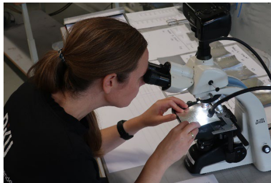
Figure 2-4 Visual observations of damage to the textile were made and photographed using a camera (1x zoom) and using a microscope (4x) with camera.
