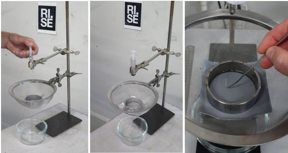
Figure 2-3 The water exposure procedure: the textile was placed on a sieve, held in place with a metal ring, with the heat exposed side facing upwards. First adding of water (left), then waiting 5 minutes and observing any water penetration (centre), and finally scratching on the side facing upwards (right).
