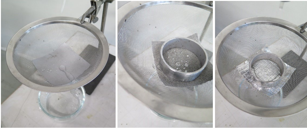
Figure A9 Water exposure set-up modifications. Version 1 (left) with textile placed in sieve. Version 2 (center) with metal ring placed gently onto the textile. Version 3 (right) with metal ring placed firmly onto the textile.
