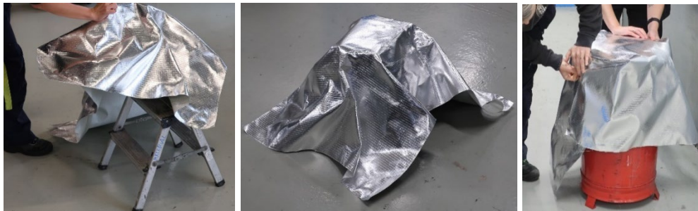
Figure 3-14 Photos from the study of handling properties of the welding protection textile, with throwing and wrapping around a small object (0.5 m high, left/centre) and an intermediate sized object (1 m high, right).
