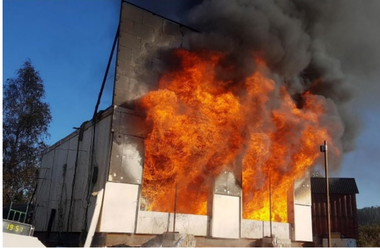
Figure A36. Photo from test 1 of full-scale mass timber buildings setting an upper boundary of the incident radiant heat to the timber façade. From Sjöström et al (2023).
