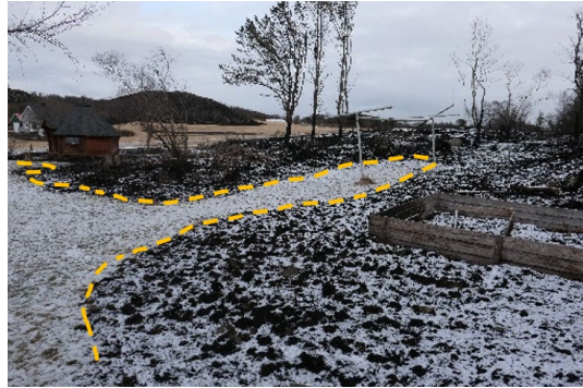
Figure A20. Charring on the ground, except for the area where the robot lawn mower had cut the grass (outlined in yellow). Photo: RISE Fire Research.
