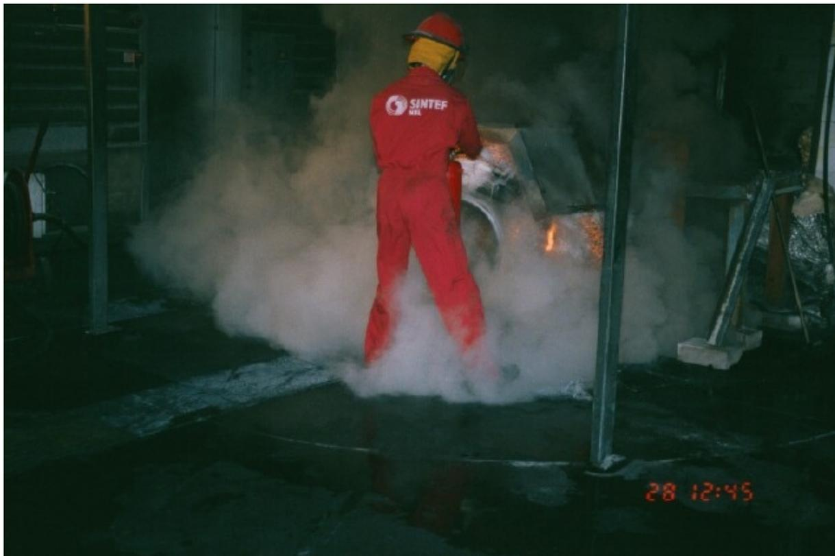
*Figure C.9: At the end of fire fighting with a dry powder fire extinguisher.*
