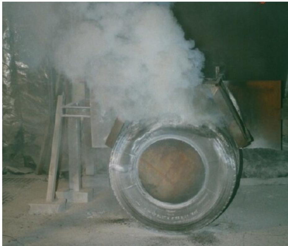
*Figure C.11: After the fire is not permanently extinguished with a dry powder fire extinguisher. There is still a certain smoke production from the tyre and one can hear crackling from the tyre. After some time there was a reflash in the tyre.*
