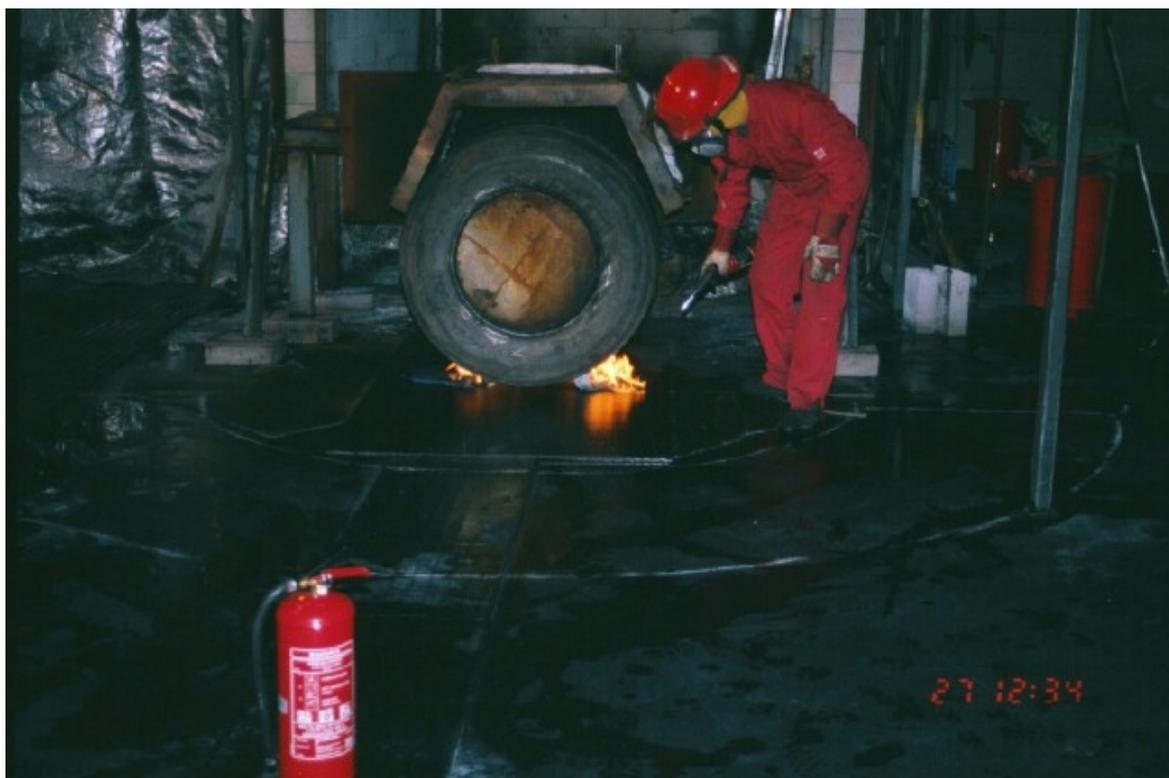
*Figure C.5: Ignition of the heptane soaked rags under the tyres.*
