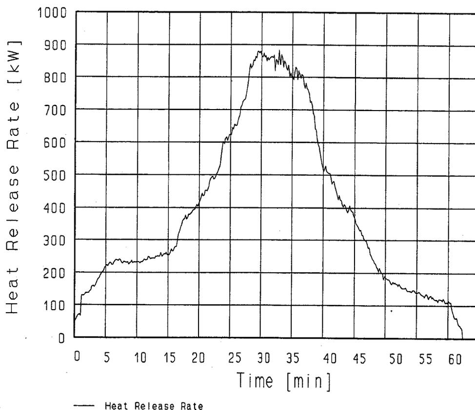
Figure A.1: The heat release rate (in kW) during a twin tyre fire. Maximum heat release rate was 878 kW. The time is given from pilot ignition of the tyres /8/.
